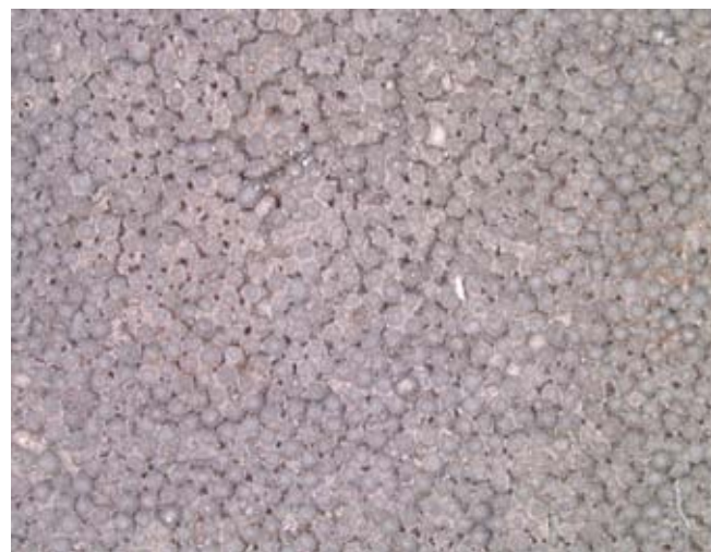
Fig. 3 Test coupon for smooth surface impingement test (13.28X; average bump diameter \sim 0.25 mm)
