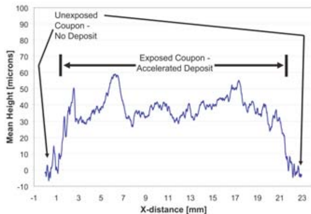
Fig. 5 23 mm long average surface trace across accelerated deposit test coupon. Vertical scale (units are microns) exaggerated for clarity. 1 mm on either end of trace is unexposed surface with no deposits.
