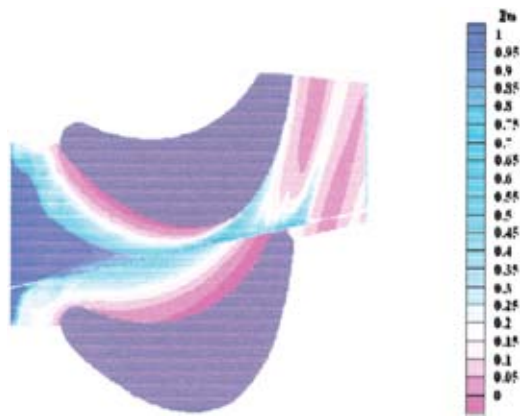
Fig. 12 Computational predictions for 1.5% front and aft slot flow and 0.25% featherseal flow
